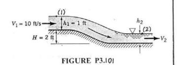
$$\frac{f_{1}}{\delta} + \frac{V_{1}^{2}}{2g} + Z_{1} = \frac{f_{2}^{2}}{\delta} + \frac{V_{2}^{2}}{2g} + Z_{2} \quad \text{where } \rho_{1} = 0, \ \rho_{2} = 0, \ Z_{1} = 3ft,$$
