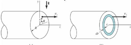
Consider a 10-mm-diameter horizontal tube through which ethyl alcohol is flowing with a steady mean velocity 0.15 m/s as is shown in the above figure. The velocity distribution is
