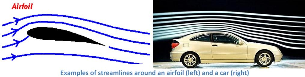
Examples of streamlines around an airfoil (left) and a car (right)
