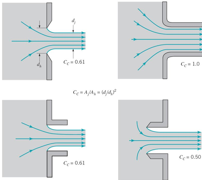
**Figure 3.14 Typical flow patterns and contraction coefficients**
