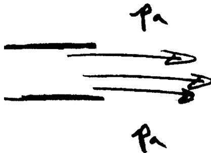
at an exit into the atmosphere jet pressure must be  $p_a$
