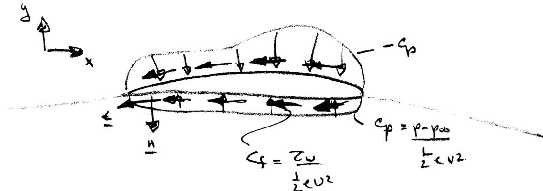
$$C_D = \frac{1}{\frac{1}{2} \rho V^2 A} \left\{ \underbrace{\int_S (p - p_\infty) \underline{n} \cdot \hat{i} dA}_{C_{Dp}} + \underbrace{\int_S \tau_w \underline{t} \cdot \hat{i} dA}_{C_f} \right\}$$
