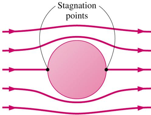
(a) Potential flow over a stationary cylinder
