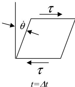
Fluid deforms, i.e., undergoes rate of strain  $\dot{\theta}$  due to shear stress  $\tau$
