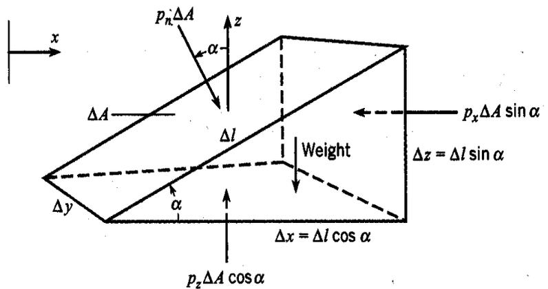
$$\begin{aligned} \Sigma F_x &= 0 \\ p_n \Delta A \sin \alpha - p_x \Delta A \sin \alpha &= 0 \\ p_n &= p_x \end{aligned}$$
