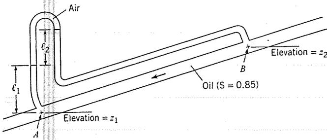
3.49 Determine (a) the difference in pressure and (b) the difference in piezometric head between points A and B. The elevations  $z_A$  and  $z_B$  are 10 m and 11 m, respectively,  $l_1 = 1$  m, and the manometer deflection  $l_2$  is 50 cm.
