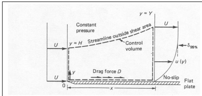
Boundary-layer thickness arbitrarily defined by  $y = \delta_{99\%}$  (where,  $\delta_{99\%}$  is the value of  $y$  at  $u = 0.99U$ ). Streamlines outside  $\delta_{99\%}$  will deflect an amount  $\delta^*$  (**the displacement thickness**). Thus the streamlines move outward from  $y = H$  at  $x = 0$  to  $y = Y = \delta = H + \delta^*$  at  $x = x_1$ .
