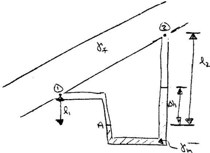
$$p_1 + \gamma_f l_1 - \gamma_m \Delta h - \gamma_f (l_2 - \Delta h) = p_2$$
