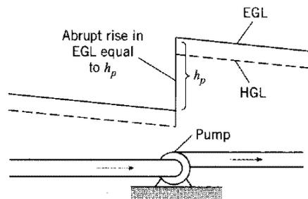
$$\frac{p_1}{\gamma} + z_1 + \frac{V_1^2}{2g} = \frac{p_2}{\gamma} + z_2 + \frac{V_2^2}{2g} + h_L$$
