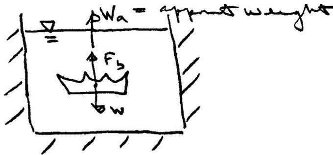
$$\sum F_{\text{vert}} = 0 = W_a + F_b - W = 0 \Rightarrow W_a = W - F_b = (\gamma_c - \gamma_w)V$$
