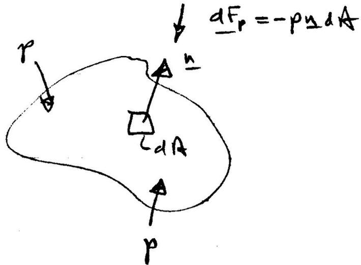
For a plane surface  $\underline{n} = \text{constant}$  such that we can separately consider the magnitude and line of action of  $\underline{F}_p$ .
