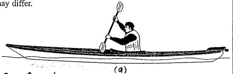
For a flat plate  $D = \frac{1}{2} \rho U^2 C_{Df} A$  where  $A = 17 \text{ ft}(2 \text{ ft}) = 34 \text{ ft}^2$  and  $C_{Df}$  is a function of  $Re_L = \frac{UL}{\nu}$  (1)
