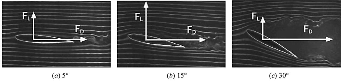
Variation of the lift-to-drag ratio with angle of attack:
