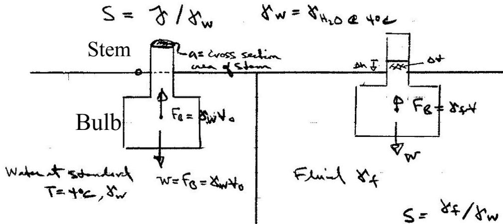
$$W = mg = \gamma_f V = S \gamma_w V$$
