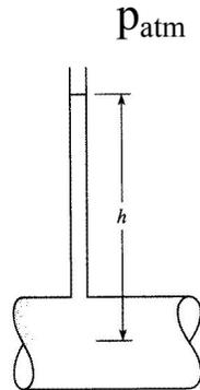
$$p_{\text{atm}} + \gamma h = p_{\text{pipe}} = p \quad \text{absolute}$$
