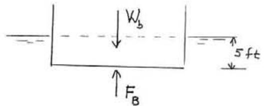
$W_b \sim$  weight of barge (unloaded)
