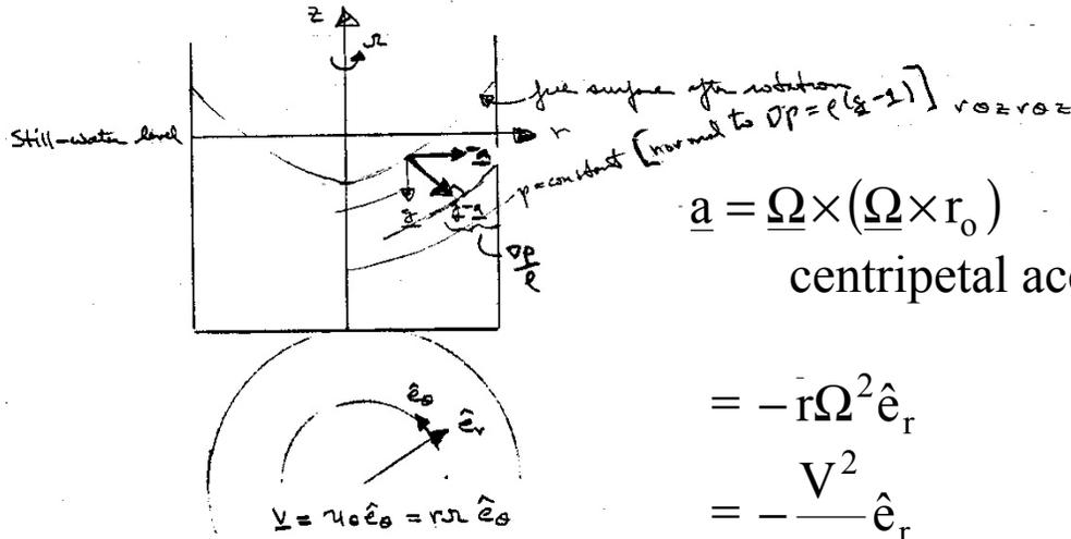
$$\underline{a} = \underline{\Omega} \times (\underline{\Omega} \times \underline{r}_0)$$
