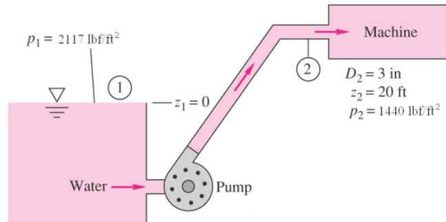
$$\frac{p_1}{\gamma} + \alpha_1 \frac{V_1^2}{2g} + z_1 = \frac{p_2}{\gamma} + \alpha_2 \frac{V_2^2}{2g} + z_2 - h_p + h_f$$
