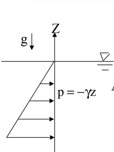
$$\frac{\partial p}{\partial z} = -\rho g = -\gamma \quad \rho = \text{constant for liquid}$$
