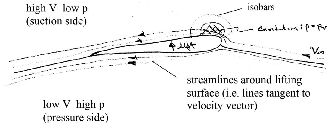
$$\text{Cavitation number} = \frac{p - p_v}{\frac{1}{2} \rho V_\infty^2}$$
