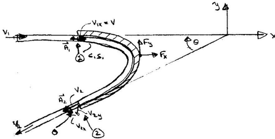
CV and CS are for jet so that  $F_x$  and  $F_y$  are vane reactions forces on fluid
