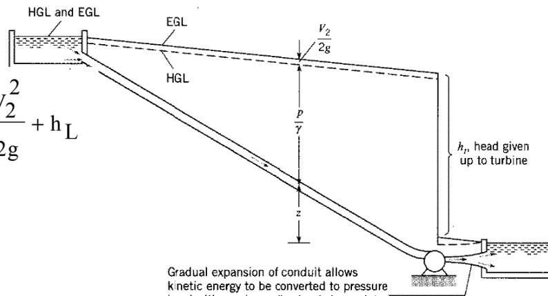
Gradual expansion of conduit allows kinetic energy to be converted to pressure head with much smaller  $h_L$  at the outlet; hence the HGL approaches the EGL.
