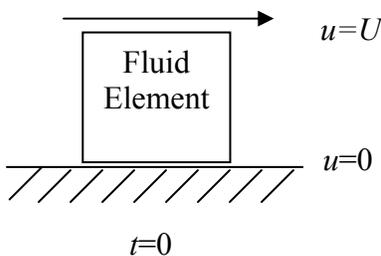
No slip condition: no relative motion between fluid and boundary, i.e., fluid in contact with lower plate is stationary, whereas fluid in contact with upper plate moves at speed  $U$ .
