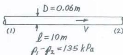
For the horizontal pipe ( $z_1 = z_2$ ) with  $V_1 = V_2$  the energy equation
