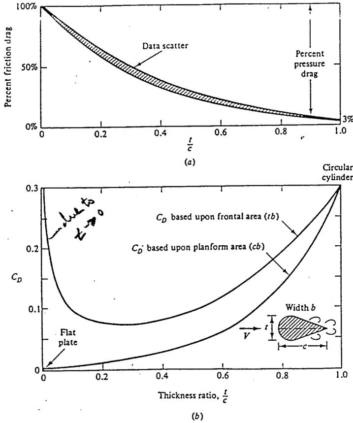
Fig. 7.12 Drag of a streamlined two-dimensional cylinder at  $Re_c = 10^6$ : (a) effect of thickness ratio on percentage friction drag; (b) total drag versus thickness when based upon two different areas.
