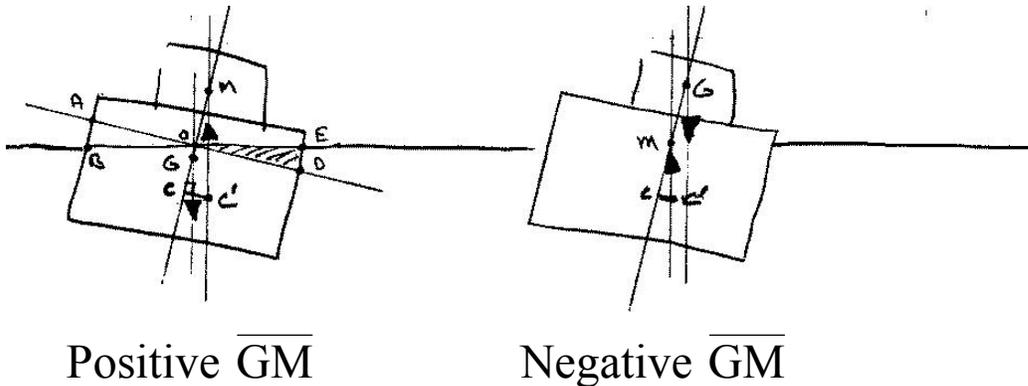
The center of buoyancy (centroid of the displaced volume) shifts laterally to the right for the case shown because part of the original buoyant volume AOB is transferred to a new buoyant volume EOD.
