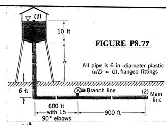
$$\frac{\rho_{1}}{b} + \frac{V_{1}^{2}}{2g} + Z_{1} = \frac{\rho_{2}}{b^{2}} + \frac{V_{2}^{2}}{2g} + Z_{2} + (f\frac{l}{D} + \Sigma K_{L}) \frac{V^{2}}{2g}, \text{ where } \rho_{1} = 0, V_{1} = 0, Z_{1} = 16ff + h,$$
