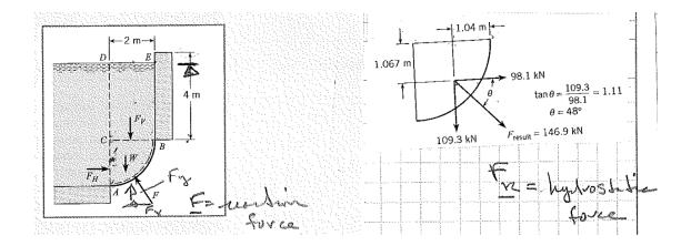
In the figure, surface AB is a circular arc with a ridius of 2m and a depth of 1m into the paper. The distance EB is 4m. The fluid above surface AB is water, and atmospheric pressure prevails on the free surface of the water and on the bottom side of surface AB. Find the magnitude and line of action of the hydrostatic force acting on surface AB.
