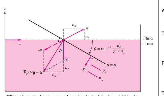
Tilting of constant-pressure surfaces in a tank of liquid in rigid-body acceleration.
