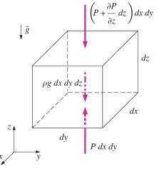
The body force and the surface pressure force acting on a differential fluid element in the vertical direction.
