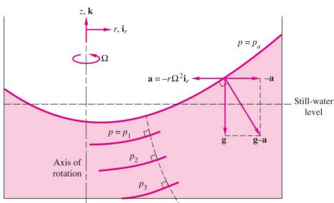
Development of paraboloid constant-pressure surfaces in a fluid in rigid-body rotation. The dashed line along the direction of maximum pressure increase is an exponential curve. 9/14/2016
