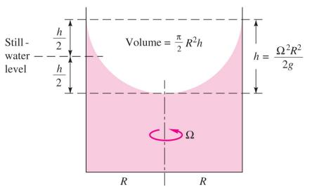
Determining the free surface position for rotation of a cylinder of fluid about its central axis.
