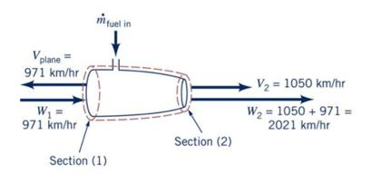
$$\frac{DB_{\rm sys}}{Dt} = \frac{d}{dt} \int_{\rm CV} \beta \rho dV + \int_{\rm CS} \beta \rho \underline{V}_r \cdot \underline{n} dA$$
