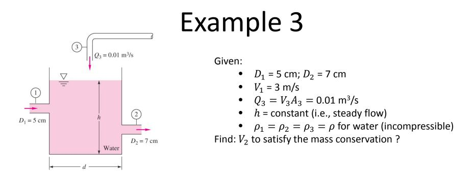
RTT for a steady and uniform flow across discrete CS:
