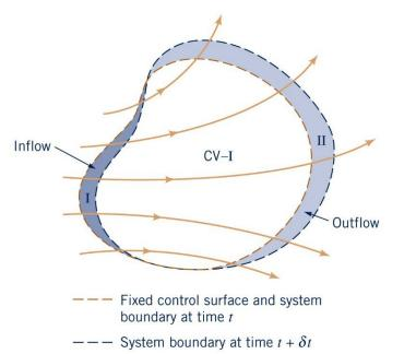
Control volume (CV) and system for flow through an arbitrary, fixed control volume
