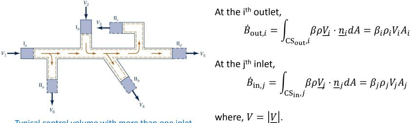
Typical control volume with more than one inlet and outlet.
