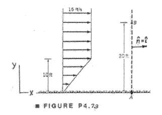
For momentum  $B = m\underline{V}$ , the intensive parameter  $b(\text{or }\beta) = B/m = \underline{V}$ . Thus, for  $CS_{out} = AB$  of unit depth,
