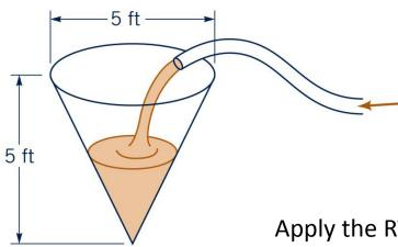
Estimate the time required to fill with water a cone-shaped container 5 ft hight and 5 ft across at the top if the filling rate is 20 gal/min.
