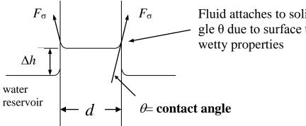
Fluid attaches to solid with contact angle  $\theta$  due to surface tension effect and
