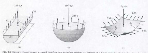
Fig. 1.9 Pressure change across a curved interface due to surface tension: (a) interior of a liquid cylinder; (b) interior of a spherical droplet; (c) general curved interface.
