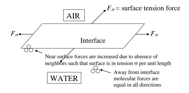
$\sigma_{air/water} = 0.073 \text{ N/m}$   $F_{\sigma} = \sigma \times L = \text{line force with direction normal to the cut}$ L = length of cut through the interface
