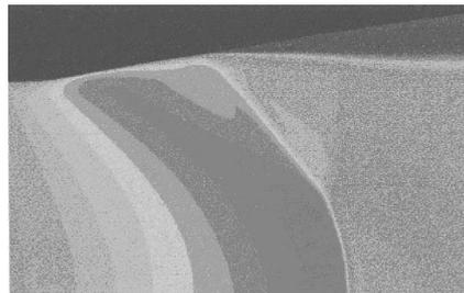
The FlowLab template for the nozzle is designed to use three meshes with varying degrees of mesh density, including boundary layer stretching. As expected, the viscous solutions show the desired  $\lambda$ -shock behaviour seen in Figure 4. It should be noted that while the FlowLab template provides adequate resolution at low pressure ratios, the template could not grid resolve solutions at high pressure ratios for the short run times desired.
