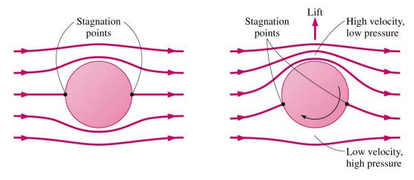
(a) Potential flow over a stationary cylinder
