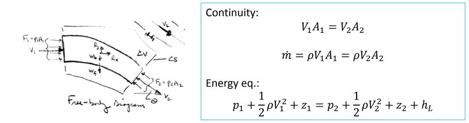
*x*-momentum:  $R_x + p_1 A_1 - p_2 A_2 \cos \theta = \underbrace{\dot{m}(V_2 \cos \theta)}_{\text{out}} - \underbrace{\dot{m}(V_1)}_{\text{in}}$
