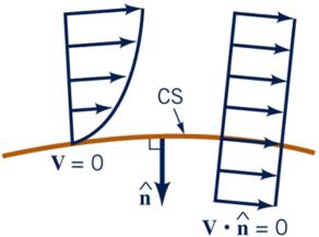
Note: Shearing forces can be avoided by carefully selecting the CV such that CS's are parallel with the flow direction.
