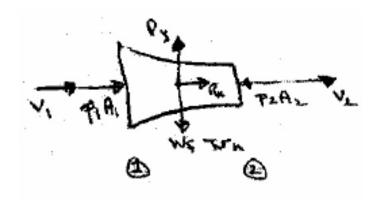
Continuity:  $V_1A_1 = V_2A_2$   $\dot{m} = \rho V_1A_1 = \rho V_2A_2$ Energy eq. with  $p_2 = 0$  and  $z_1 = z_2$ :  $p_1 + \frac{1}{2}\rho V_1^2 = \frac{1}{2}\rho V_2^2 + h_L$
