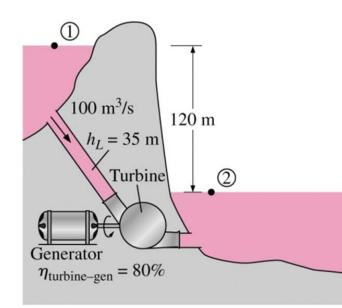
$$\frac{p_1}{\gamma} + \frac{V_1^2}{2g} + z_1 + h_p = \frac{p_2}{\gamma} + \frac{V_2^2}{2g} + z_2 + h_t + h_L$$
