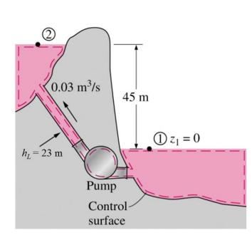
$$\frac{p_1}{\gamma} + \frac{V_1^2}{2g} + z_1 + h_p = \frac{p_2}{\gamma} + \frac{V_2^2}{2g} + z_2 + h_t + h_L$$
