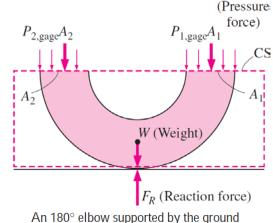
In most flow systems, the force  $\vec{F}$  consists of weights, pressure forces, and reaction forces. Gage pressures are used here since atmospheric pressure cancels out on all sides of the control surface.
