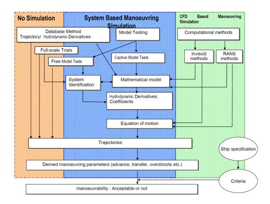
Figure 2-1 Overview of Maneuvering prediction methods (Proceedings of 25<sup>th</sup> ITTC, Vol. I, pp. 145).
