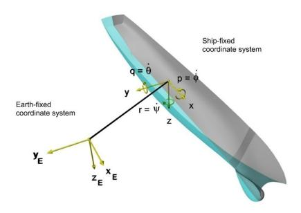
Figure 2-2 Earth- and ship-fixed coordinate systems.
