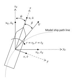
Figure 2-3 General PMM test coordinate system and motion parameters.
