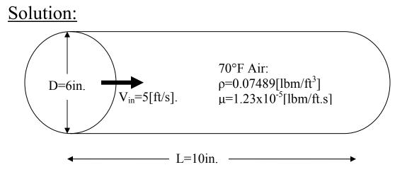
At the end of the test section, local Reynolds number is computed as;
