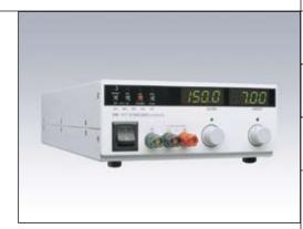
The XHR is power factor corrected for low current draw — only 11 amps at 120 volts AC for 1000 watts — and reduced generation of input current harmonics. Zero voltage or "soft switching" virtually eliminates switching transients for high efficiency, low noise and high reliability. It is also stackable, with a small footprint, front panel binding post connectors, and a low current requirement with universal input, making the XHR ideal for benchtop applications.
