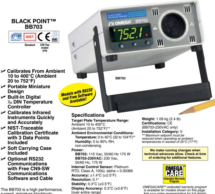
rugged, miniature blackbody calibrator. It is used for infrared pyrometer calibrations with a temperature range of ambient 10 to 400°C (ambient 20 to 752°F). With its unique miniature design and built-in 29 mm (1.125") target plate, the BB703 is an ideal and economical infrared calibrator for any laboratory or field service application. The "-C2" option allows for remote configuring, adjustment, and reading. Free software is included with these models.
