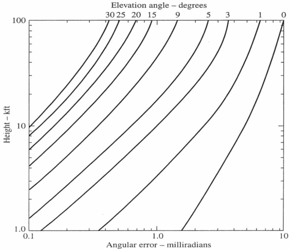
**Calculated angle error (abscissa) due to atmospheric refraction for a standard atmosphere as function of elevation angle and target height (ordinate)**
