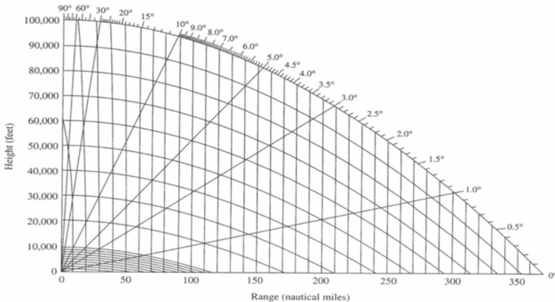
**Radar range-angle-diagram used to plot antenna coverage, based on exponential model of refraction with  $k = 313$ .**
