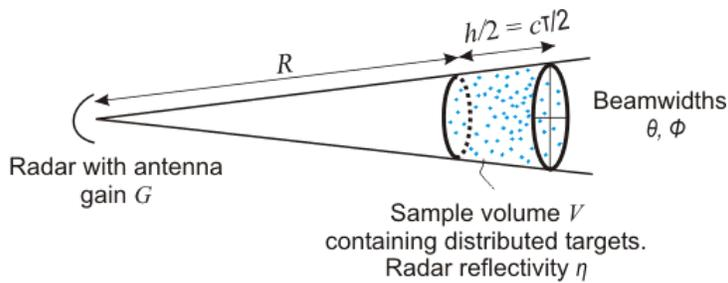
$$V_1 = \pi \frac{R \theta}{2} \frac{R \phi}{2} \frac{h}{2} \quad (\text{general})$$
