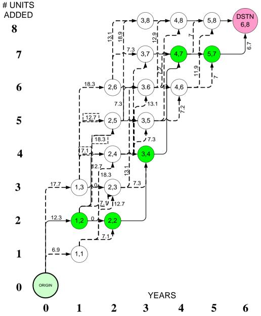
Shown on the left is the **shortest path** from the initial node to the destination, node (6,8).
