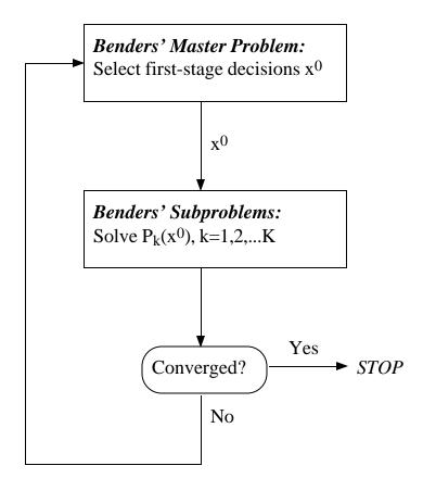
In either the Lagrangian relaxation approach or Benders' decomposition, the burden of the computation lies in the respective master problems: searching for the optimal  $\lambda$  in the case of Lagrangian relaxation, & searching for the optimal  $x^0$  in the case of Benders' decomposition.
