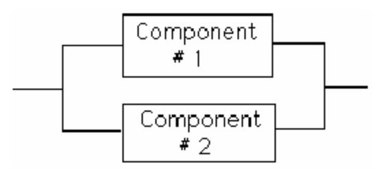
*Example*: a 2-engine plane fails only if *both* of its engines fail.
