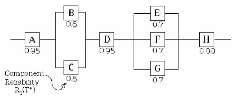
Decompose the system into series &/or parallel subsystems:
