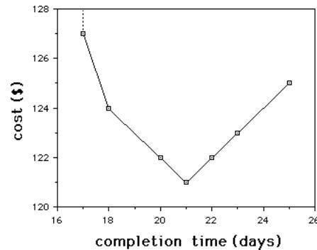
Using the output of parametric analysis, we can plot the objective vs. the project duration!
