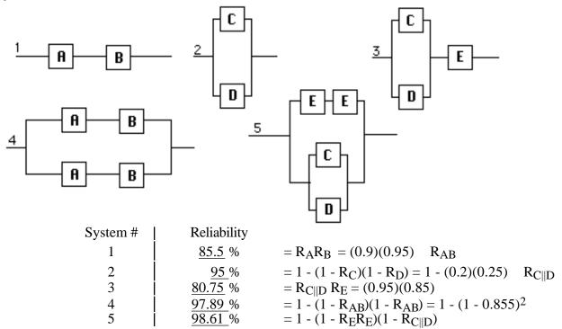
Note that the reliability is found by subtracting the above failure probabilities from 1.0. Thus,  $R_A=90\%$ ,  $R_B=95\%$ ,  $R_C=80\%$ ,  $R_D=75\%$ , and  $R_E=85\%$ .
