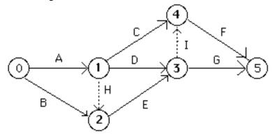
c. The activity durations (in days) are given below on the arrows. Compute the Early Times (ET) and Late Times (LT) for each node, writing them in the box (with rounded corners) beside each node.
