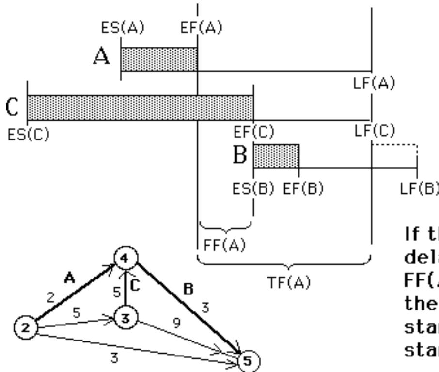
If the start of A is delayed by more than FF(A), the "free float", then B cannot be started at its early start time, ES(B)
