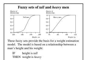
The value of the output or a truth membership grade of the rule consequent can be estimated directly from a corresponding truth membership grade in the antecedent. This form of fuzzy inference uses a method called monotonic selection.
