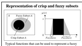
set are sigmoid, gaussian and pi. However, these functions increase the computation time. Therefore, most applications use linear fit functions.
