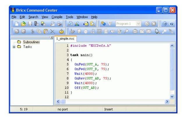
The interface looks like a standard text editor, with the usual menu, and buttons to open and save files, print files, edit files, etc. But there are also some special menus for compiling and downloading programs to the robot and for getting information from the robot. You can ignore these for the moment.
