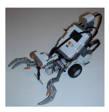
We also need the test pad with the black track that comes with the NXT set. The basic principle of line following is that the robot keeps trying to stay right on the border of the black line, turning away from line if the light level is too low (and sensor is in the middle of the line) and turning towards the line if the sensor is out of the track and detects a high light level. Here is a very simple program doing line following with a single light threshold value.
