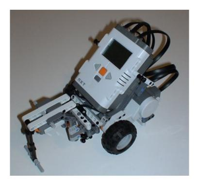
Connect the touch sensor to input 1 on the NXT.
