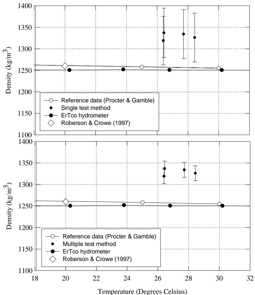
Figure 9. Density of 99.7% aqueous glycerin solution test results and comparison with benchmark data
