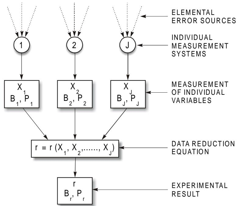
Figure 3. Propagation of errors into experimental results (AIAA, 1995)
