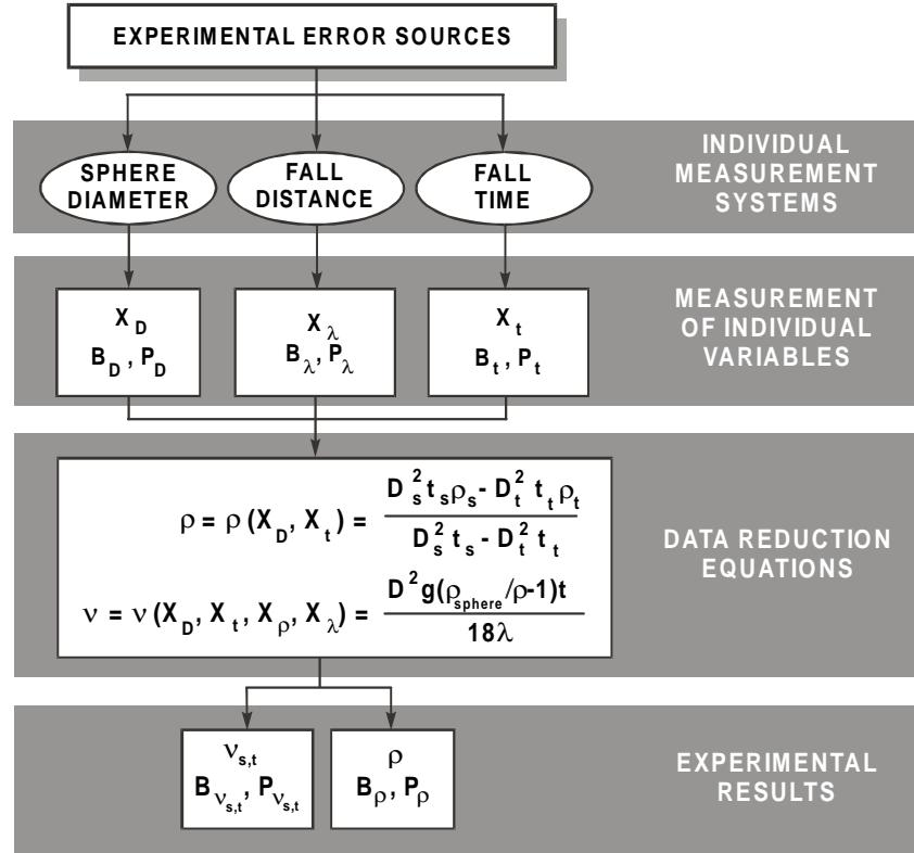
Figure 8. Block diagram of experiment
