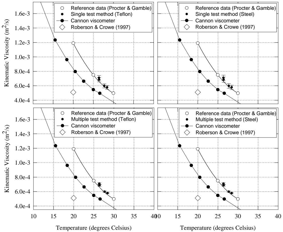
Figure 10. Kinematic viscosity of 99.7% aqueous glycerin solution test results and comparison with benchmark data
