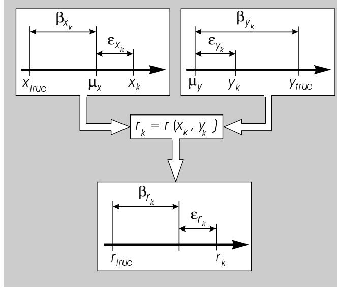
Figure 6. Propagation of bias and precision errors into a two variable result
