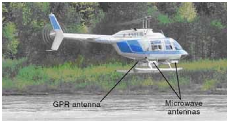
Helicopter-mounted radar experiment. Two microwave antennas are located just below the cabin on each side. The radar antenna is the large white structure below the helicopter.
