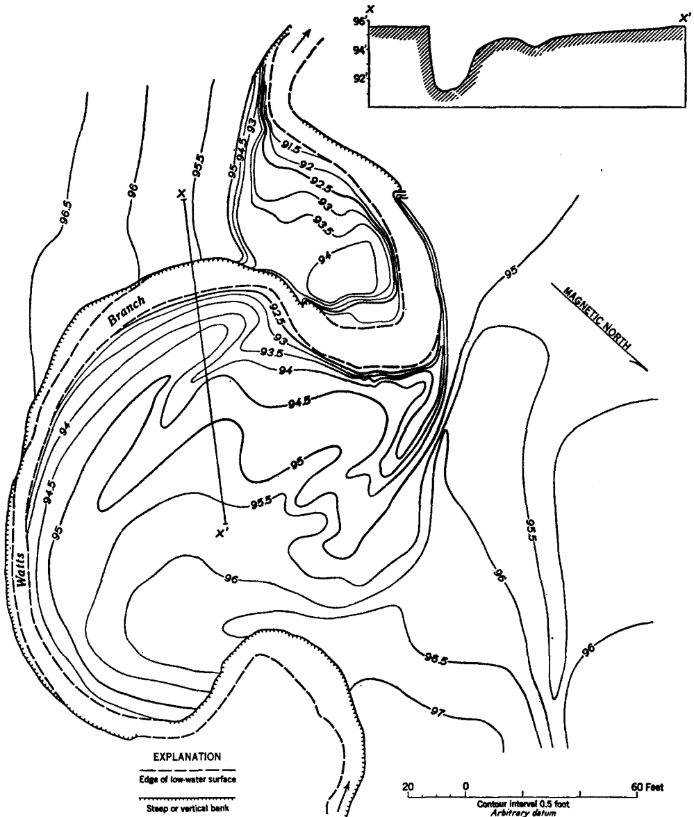
FIGURE 7.—MAP AND CROSS SECTION OF A TYPICAL POINT BAR OF THE FLOOD PLAIN OF WATTS BRANCH, 1 MILE NORTHWEST OF ROCKVILLE, MARYLAND After Wolman and Leopold (1957)
