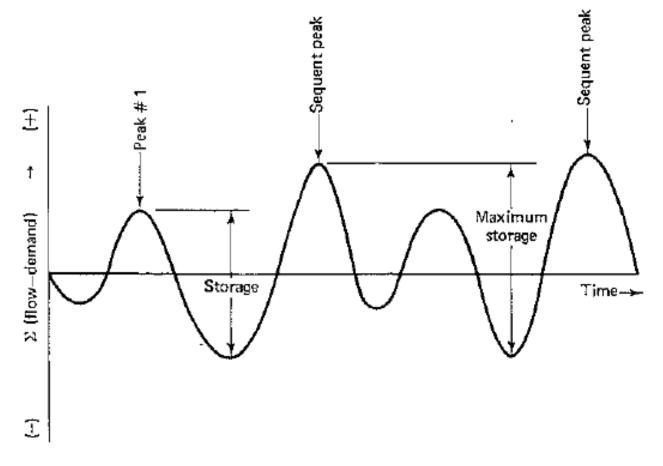
FIGURE 7.5 Illustration of sequent-peak algorithm.
