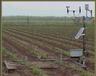
Continuous weighing of soil and water in the device
