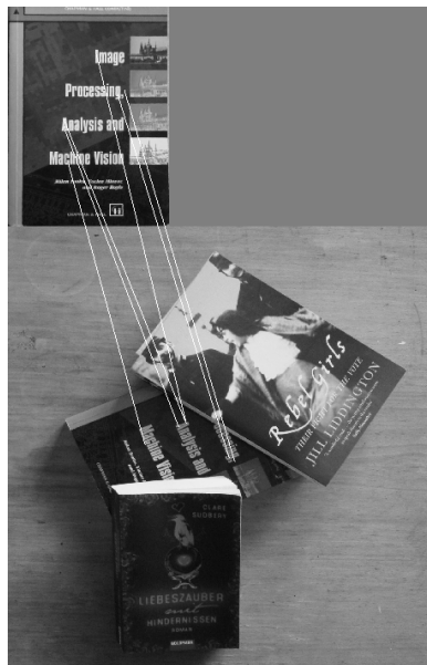
Figure 8.5: Location by SIFT of 6 point matches in a challenging image, 5 of which are correct.
