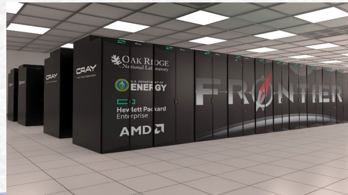
Supercomputer FRONTIER, DOE/SC/Oak Ridge National Laboratory, Peak Compute: 1,679.82 (PFlop/s), TOP500: 1st, June 2022-2023
