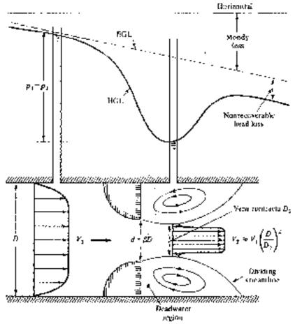
The flow in the basic duct of diameter D is forced through an obstruction of diameter d; the  $\mathbf{b}$  ratio of the device is a key parameter,  $\mathbf{b} = d/D$ . Applying Bernoulli and continuity equations for incompressible steady frictionless flow, and then calibrating the device we can get a relationship between the discharge Q and the pressure change  $(p_1-p_2)$  in the form
