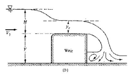
For certain simple geometry channels, the discharge Q correlates with the blockage height (the head H on the weir) to which the upstream flow is deflected in the presence of the weir through a relationship of the form
