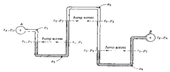
By repeated application of the hydrostatic formula we can relate the pressures  $p_A$  and  $p_B$  to the densities and the levels of the fluid levels in the tubes. Usually the central columns are placed on the sides of the same guide bar. Separate slides are provided for each column, and the graduated scale is fixed to one and read by the vernier on the other as shown in Figure 2.
